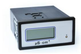
The MA48LWD is a high-resolution conductivity measurement and display device. It is equipped with a digital display and a potentiometer for cell adjustment. The compact design according to DIN IEC 61554 is made of flame-retardant noryl and designed for panel mounting. The device is connected by screw-type connectors on the back side.
